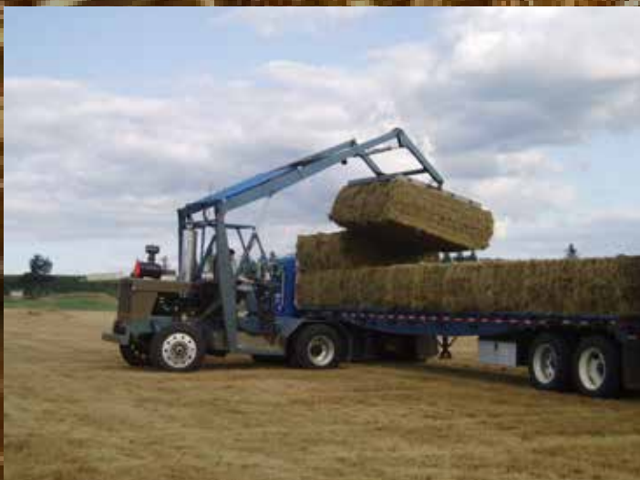
The bale loader picks up two bales of straw at a time and loads them onto the trailer. Each bale weighs between 1100 and 1300 pounds depending on the crop.
